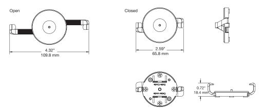
One55/One65/One60 2 Arm Bracket Plate with tablet brackets (DBT282):
