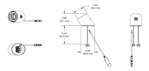
OnePOD Non Connected Recoiler Standard Cable (DBD300):
