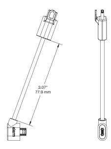
One55/One65/One60 Tablet USB Micro Power Connector (DBT500):
