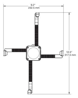
Tablet Bracket Arm Range: Width: 5.8" – 9.2" (146.5 mm – 232.5 mm) Height: 8.6" – 12.5" (218.5 mm – 317.5 mm)
