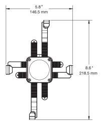
Handheld Bracket Arm Range: Width: 3.0" – 5.8" (77.1 mm – 146.5 mm) Height: 5.4" – 8.6" (136.5 mm – 218.5 mm)
