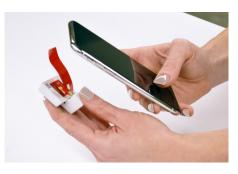
Within the InVue LIVE app, use the camera on your device to scan the code and enroll the sensor. Fill out the information for the sensor and the device that will be displayed.
