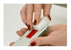
Plug the power connector on the sensor into the device.
